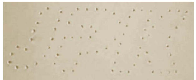
Figure 3 1 \mu\text{m} silica beads in multiplexed traps. 80 particles are trapped simultaneously and arranged to form the JPK company logo. Ultrafast AODs allow the parallel trapping and manipulation of hundreds of particles.
