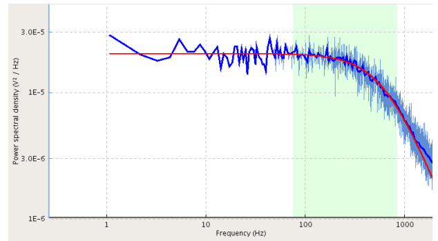
Figure 7 Power spectrum derived from the isolated signal of one of the traps in Figure 4. After clean separation of the noise signals, power spectrum-based calibration is possible for each trap. The red line is a Lorentzian curve fitted to the data in the range highlighted in green. It is used to determine the corner frequency and to calculate detection sensitivity and trap stiffness.
