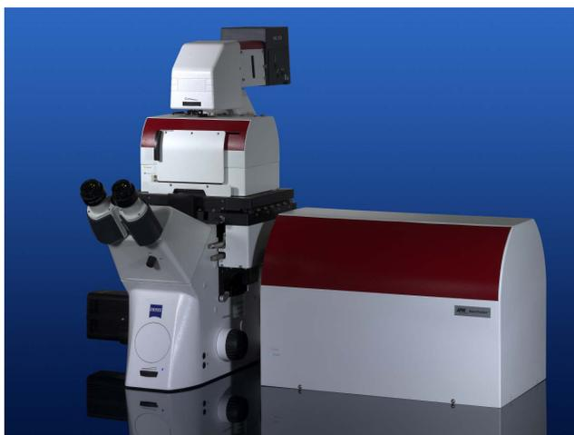
*Figure 1: The NanoTracker™ optical tweezers platform.*
