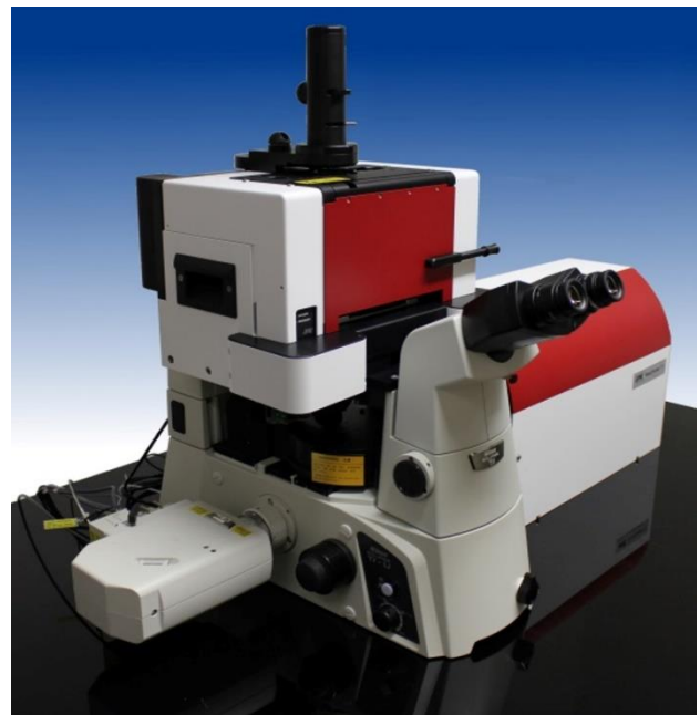
Fig. 1: Dual-trap optical tweezers NanoTracker™ 2 combined with Nikon's laser scanning confocal microscope.
