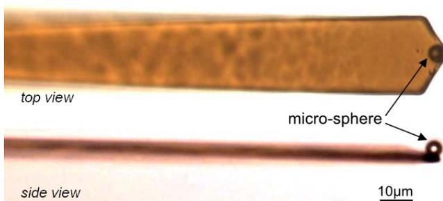
**Fig. 2:** Cantilever with 5  $\mu$ m micro-sphere attached at the end of the cantilever beam. Using the new deposition procedure, the location of the micro-sphere can be easily adjusted until the
