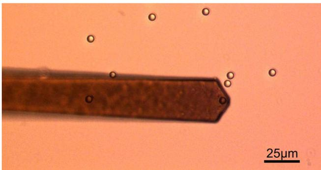
**Fig. 1:** Tipless cantilever in water with 5  $\mu\text{m}$  micro-spheres
