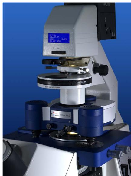
**Fig. 1:** CellHesion 200 head and Life Science stage mounted on Zeiss Axiocvert 200 with light transmission condenser for Phase contrast and DIC illumination.
