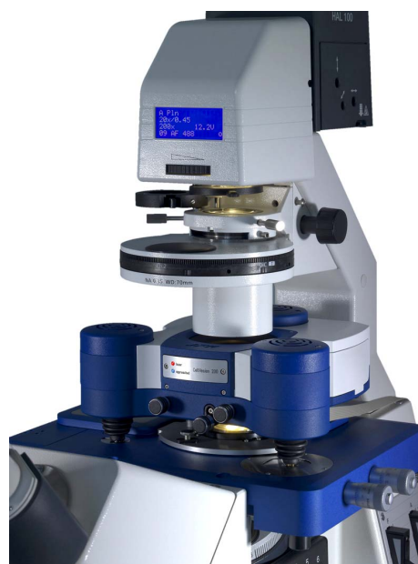
Fig. 1: CellHesion 200 head and Life Science stage mounted on Zeiss Axiovert 200 with light transmission condenser for Phase contrast and DIC illumination.
