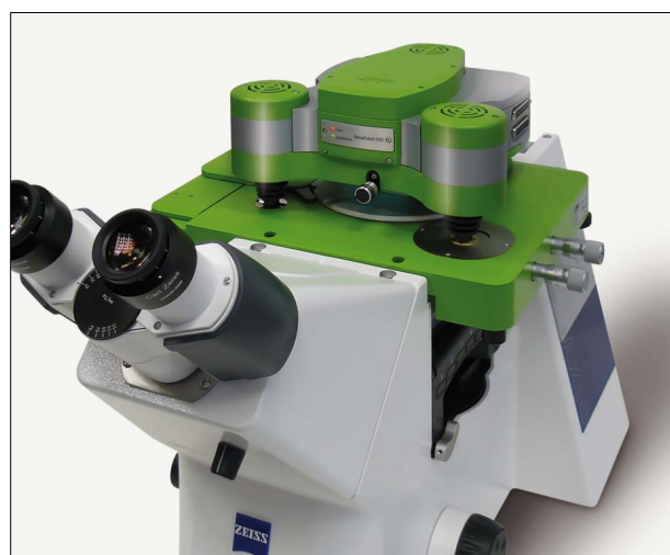
Fig.1: ForceRobot® 300 mounted on an inverted microscope including the MappingStage for automated force spectroscopy mapping.
