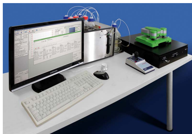
Fig. 5: ForceRobot® 300 mounted on the MappingStage including a joystick, the 8Channel FluidicsModule™ and the ForceRobot® Software.
