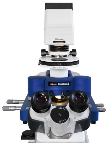
**Fig. 4:** Nanowizard 4 AFM standing on an inverted optical microscope.
