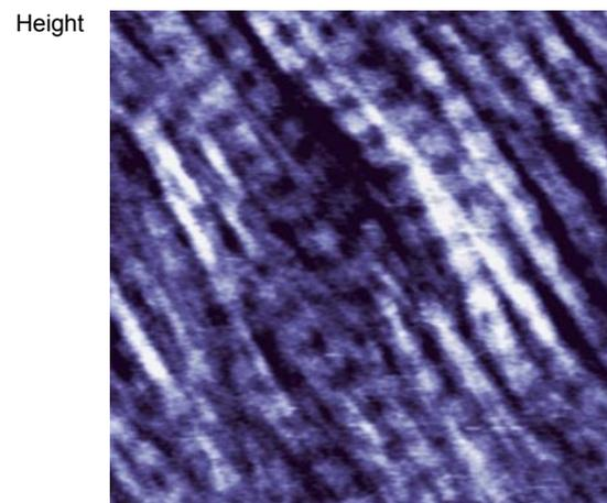
**Fig 9.** Intermittent contact mode image of unfixed collagen in buffer (750 x 750 nm, z-range 5.5 nm). Sample courtesy of A. Taubenberger, D.J. Müller Cellular Machines group, TU Dresden.
