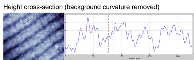
**Fig 3.** Height and vertical deflection images of a 600 x 600 nm area of a rat collagen fibril. Besides the transverse banding, there is also structure visible across the fibre, as shown in the cross-section in the lower part.
