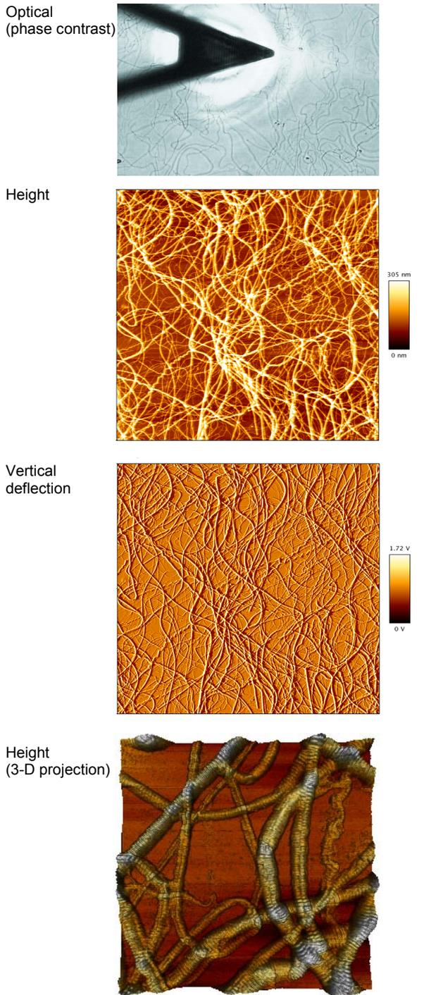
**Fig 4.** Bovine tendon collagen fibrils on APTES-glass, images courtesy of Prof. M. Horton, Bone and Mineral Center UCL and London Centre for Nanotechnology. Optical phase contrast (top), 100 x 100 micron scan area height and deflection AFM images (centre), and 5 x 5 micron 3D height image (bottom).
