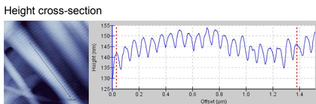
**Fig 2.** Height and vertical deflection images of a 2 x 2 micron scan area on a rat tail collagen sample. The cross-section shows 20 repeats of the D-banding marked with red lines, giving an average period of 67.3 nm.
