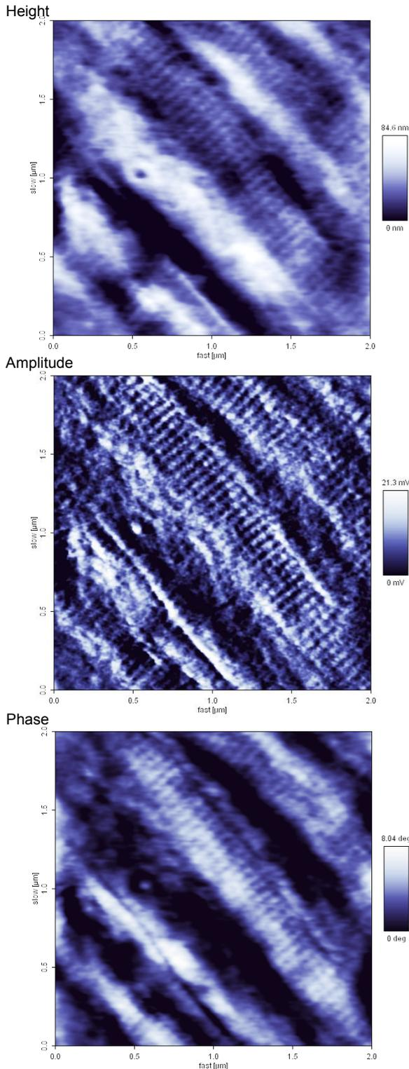
**Fig 8.** 2 x 2 micron intermittent contact mode scan of collagen-coated silicone in buffer (sample courtesy of M.J.B. Wissink, University of Twente, The Netherlands).
