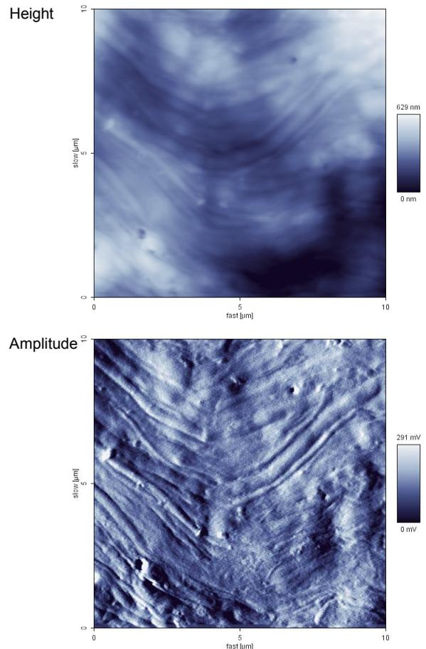
**Fig 6.** Intermittent contact mode image in liquid (10 x 10 microns) of a collagen-coated silicone film. Sample courtesy of M. J. B. Wissink, University of Twente, The Netherlands.
