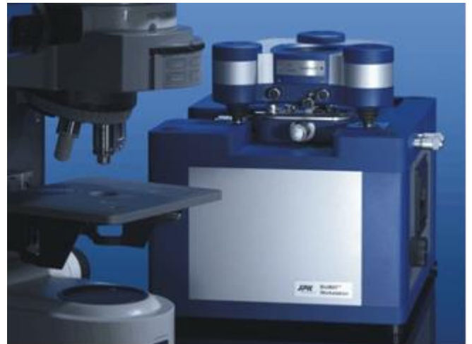
Fig. 1: NanoWizard AFM integrated into the BioMAT Workstation
