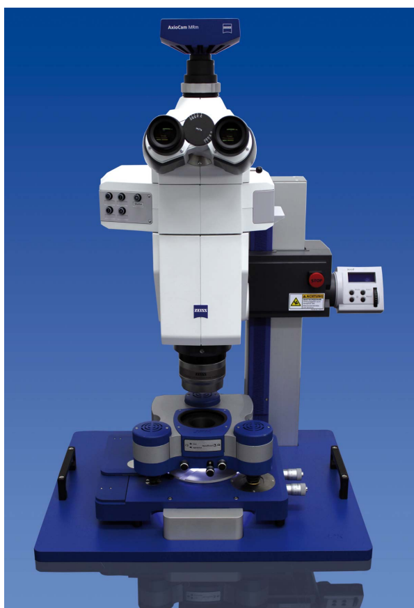
Fig. 1: The JPK NanoWizard® 3a in combination with an Axio Zoom.V16 from Zeiss
